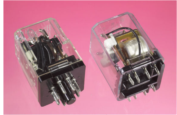
Figure 9-9. Two relays powered by 12VDC, capable of switching up to 10A at 240VAC.
