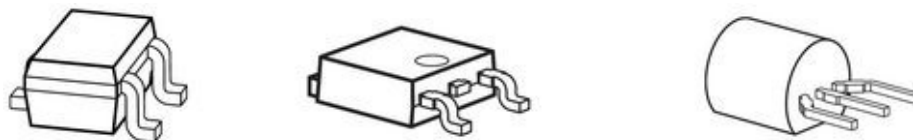
Fig. 11.19: Typical packages for BJT: two surface mount devices (SMD), small SOT-23 (left) and DPAK (TO-252, mid); TO-92 through hole device (THD, right). Package drawings by Infineon Technologies AG.
